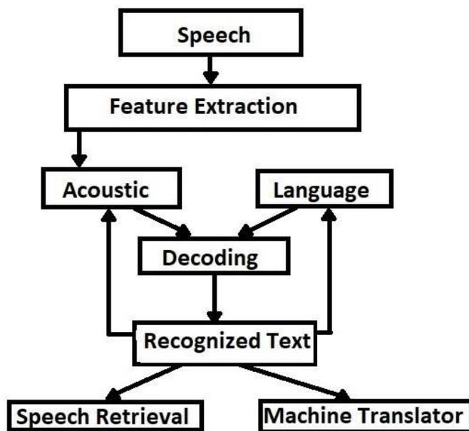
Fig2.1: Main Components of an Automatic Speech Recognition System
